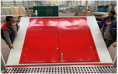
5)IN THE SAME WAY, THE DOOR PANEL IS SITTED ON THE HOPPER AND CONNECTED TO THE CORNER ELEMENTS WITH THE HELP OF PINS
