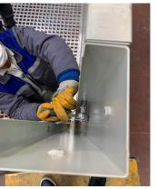
4)CORNER ELEMENTS AND PANEL ARE BOLTED AS SHOWN
